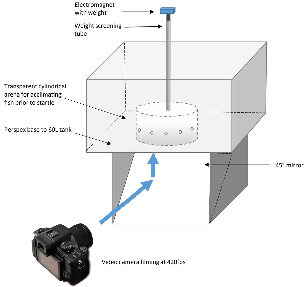
Figure S1. Experimental apparatus for testing escape responses in juvenile reef fish
