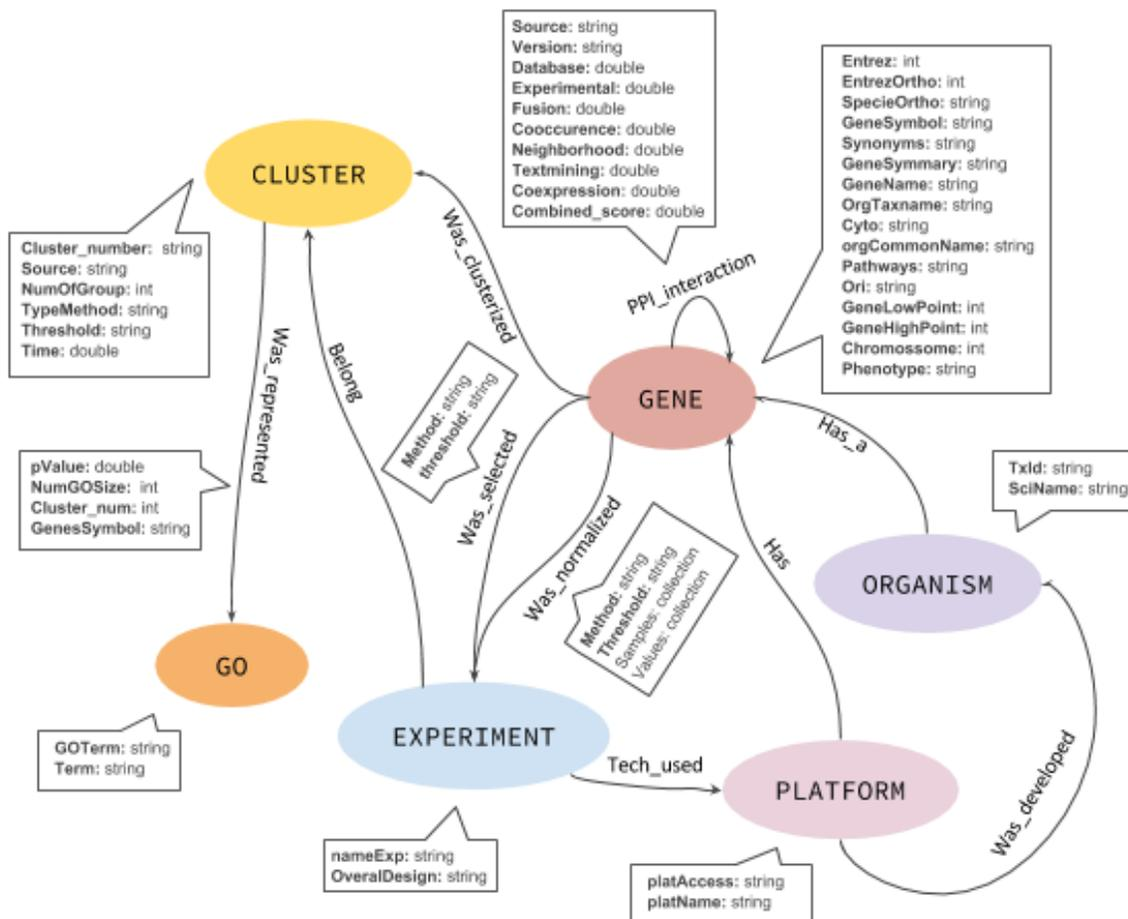
Figure 3: Figura 2: Graph database schema in GeNNet.
