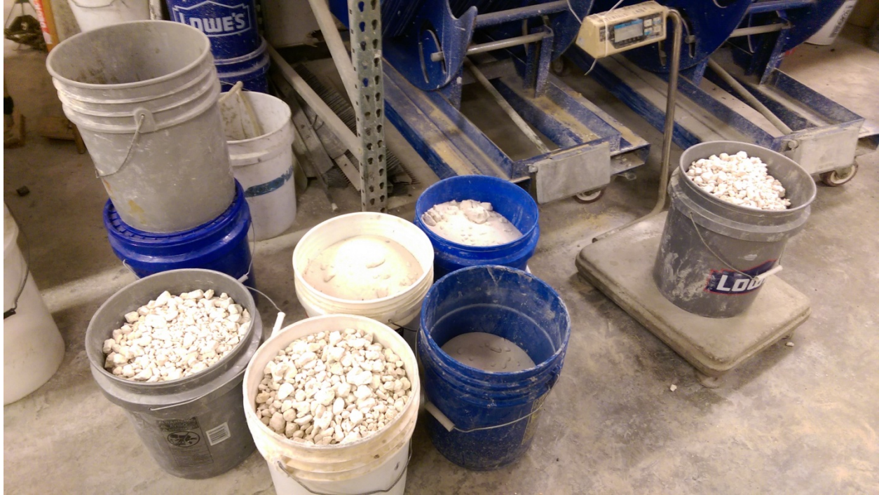
Figure S8. Batched coarse aggregate, fine aggregate and cement.
