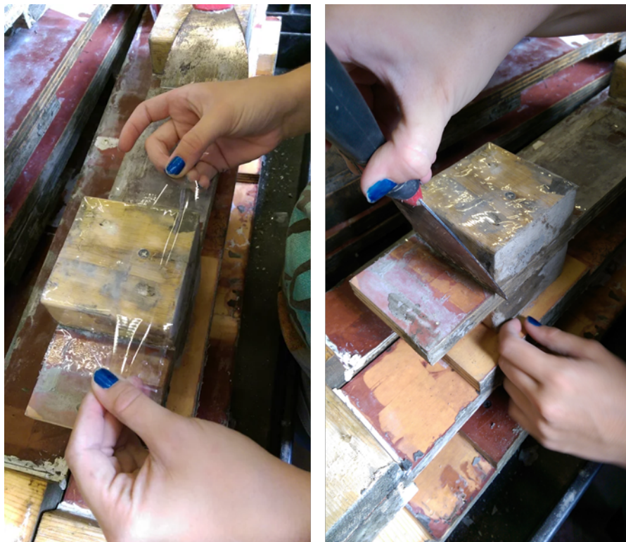
Figure S5. Apply clear packaging tape to each notch piece.
