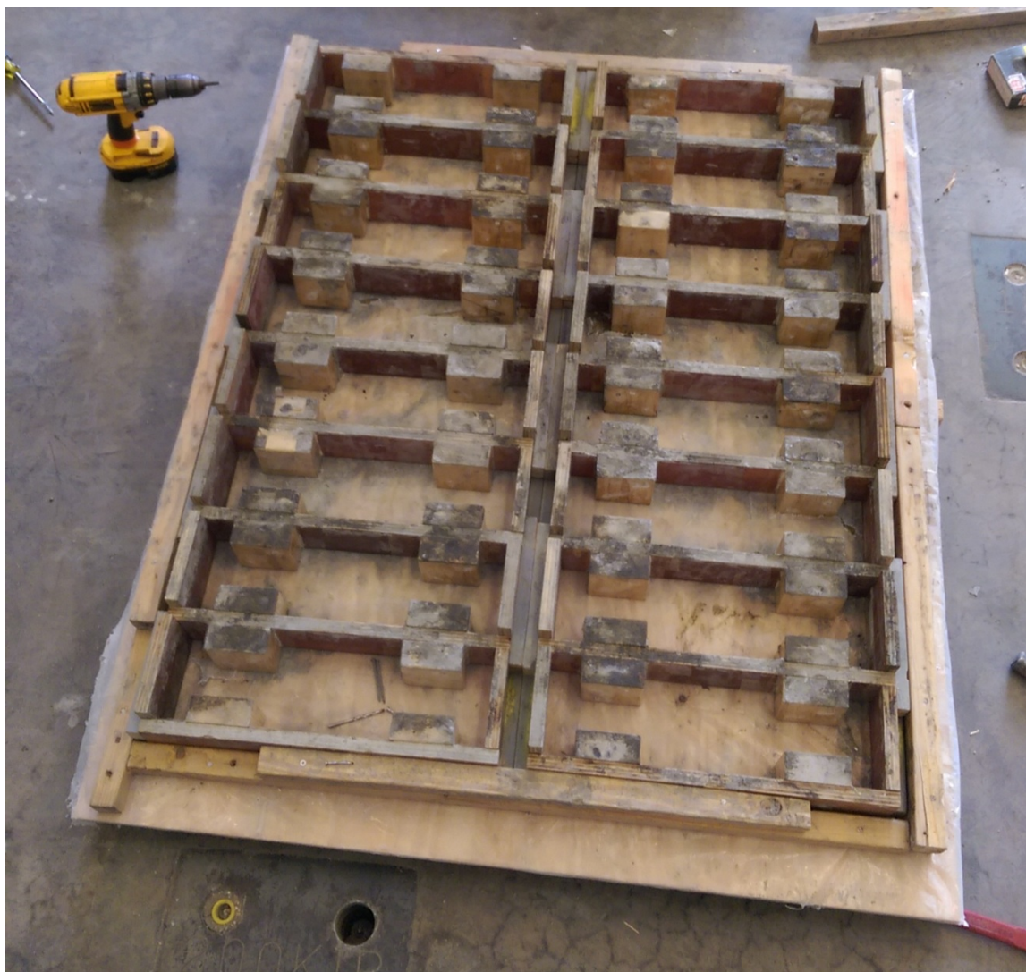
Figure S4. Two mold units for the smaller blocks fit on a single plywood base.
