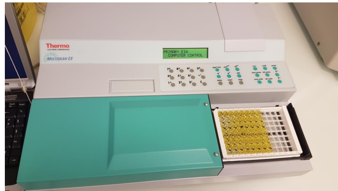
Figure 4. Spectrophotometer and coloring of the plate after addition of the stop solution.
