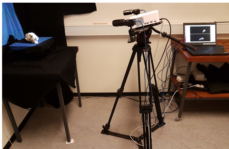
Figure 2. SeeMaLab scanner setup. Scanning a grey seal skull at the Natural History Museum in Copenhagen.
