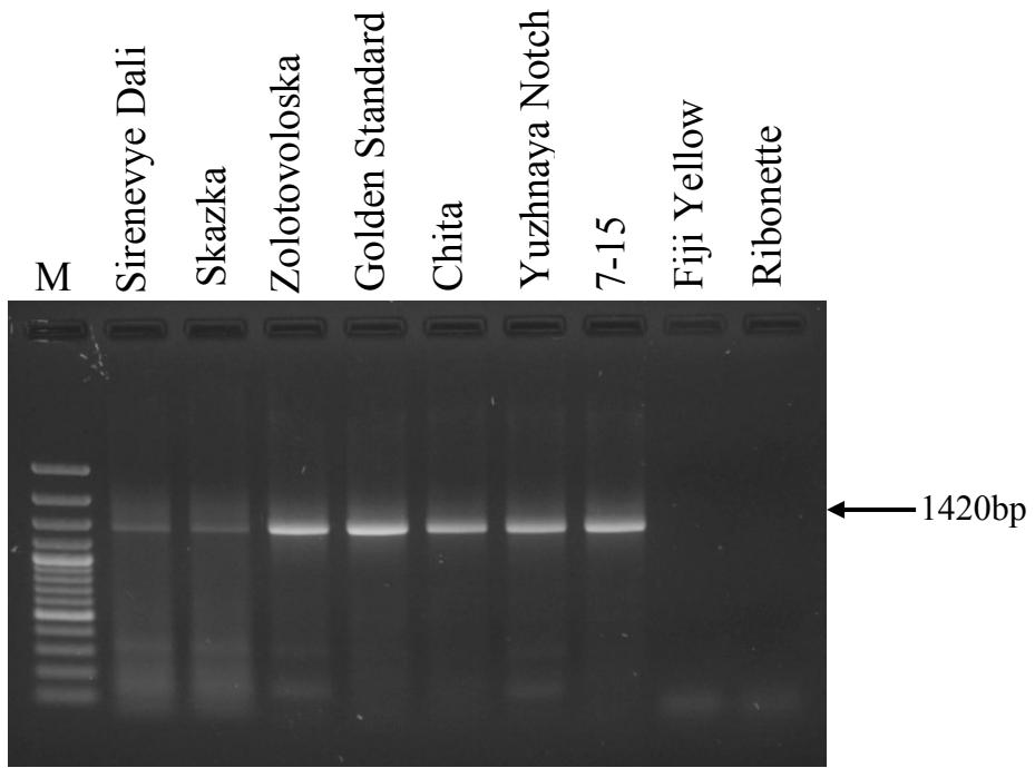
**Figure S3.** Representative analysis of RT-PCR products from chrysanthemum virus R (CVR)-infected plants by agarose gel electrophoresis. The names of chrysanthemum cultivars are indicated above the picture. M - GeneRuler 100 bp DNA ladder Plus (Thermo Scientific). The arrows to the right of the picture indicates the CVR-specific PCR products of 747, 946, and 1420 base pairs.
