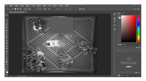
Step 4: Use "color selecting tool" to target the area for grayscale estimation (estimated grayscale is 77% in this case)
