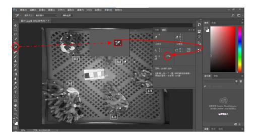
Step 5: Repeat the procedure from step 3 to 4 to estimate grayscale of standard black and white color strips (black: 80% and white: 7% in this case).
