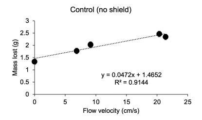
Supplemental Figure 3: Mass loss of Life Savers ™ in different flow velocities when protected by a shield or unprotected (control). Significantly less mass loss occurred behind the shield than in controls, indicating the shield effectively reduced flow velocity. Each data point is the mean mass loss of 5 Life Savers ™.
