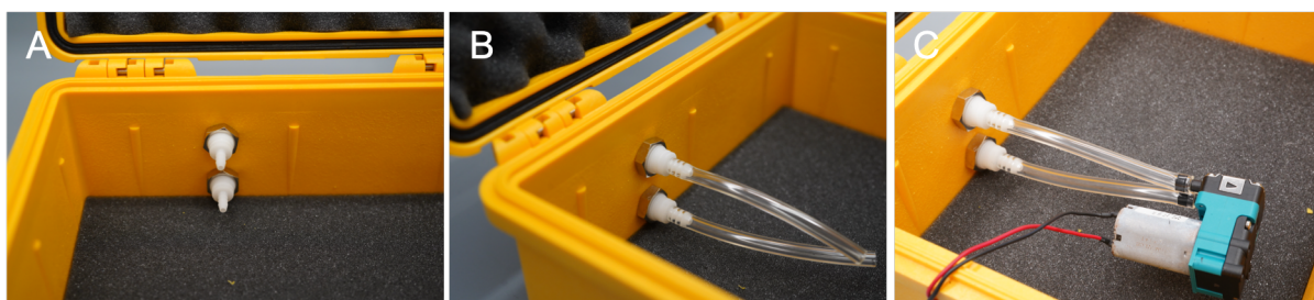
Figure 3: Connection of pump to quick-disconnect attachments
